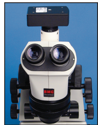
Total magnification 6.5 to 50x with 10x eyepieces 50/50 beam splitter
