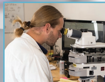
UV-vis-NIR microscopy with both transmission and incident illumination.
