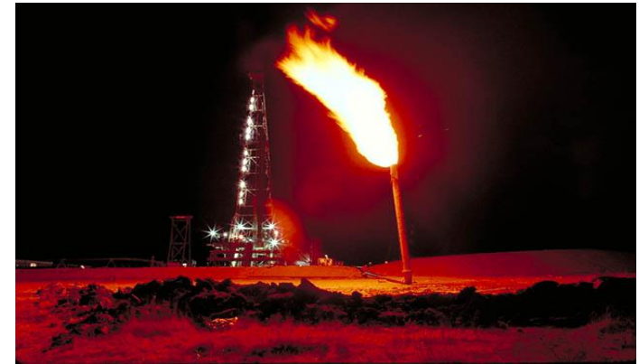
Land welltest; gas is flared off, oil stored
