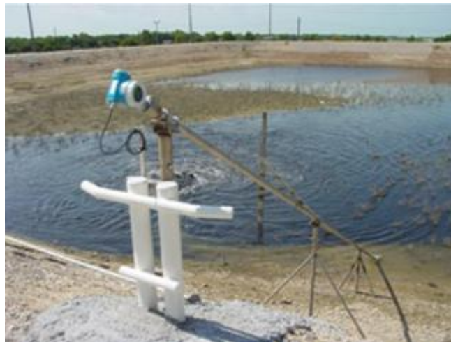
Micropilot FMR 240 installed with 30° with a 2" pipe.
